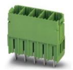
Header, Nominal current: 41 A, Rated voltage (III/2): 630 V, Number of positions: 4, Pitch: 7.62 mm, Color: green, Contact surface: Tin, Mounting: Wave soldering
