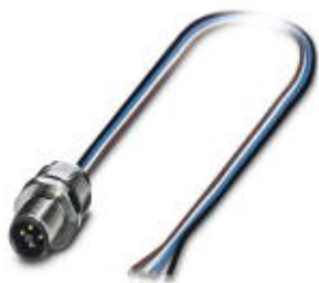
Flush-type connector, Power, 4-position, PlugLink:M12, T power, Front mounting, M16 x 1.5, Individual wires, Cable length: 0.5 m
