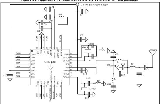
Figure 26: Application circuit: non-active DC-DC converter QFN32 package
