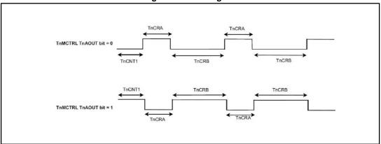
When started the first time, the TnCNT1 starts with value preprogrammed in the register and count down at the clock rate selected by the Timer/Counter 1 clock selector (TnCKC register). When an underflow occurs, the TnCNT1 is reloaded alternatively with TnCRB and TnCRB registers (in this order) and counting proceeds downward from the loaded value.
