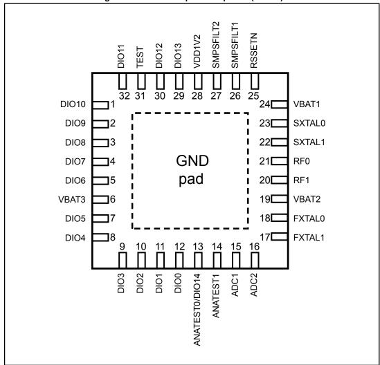
Figure 21: BlueNRG-2 pin out top view (QFN32)
