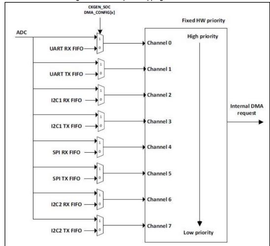
Figure 11: DMA request mapping in BlueNRG-2
