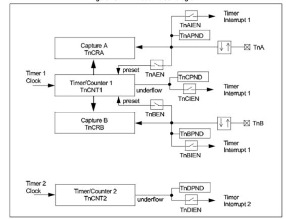
Figure 18: MFT mode 2 block diagram
