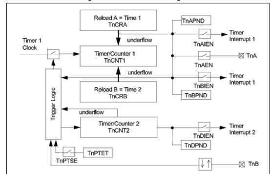
Figure 17: MFT mode 1a block diagram
