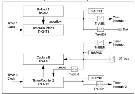
Figure 20: MFT mode 4 block diagram
