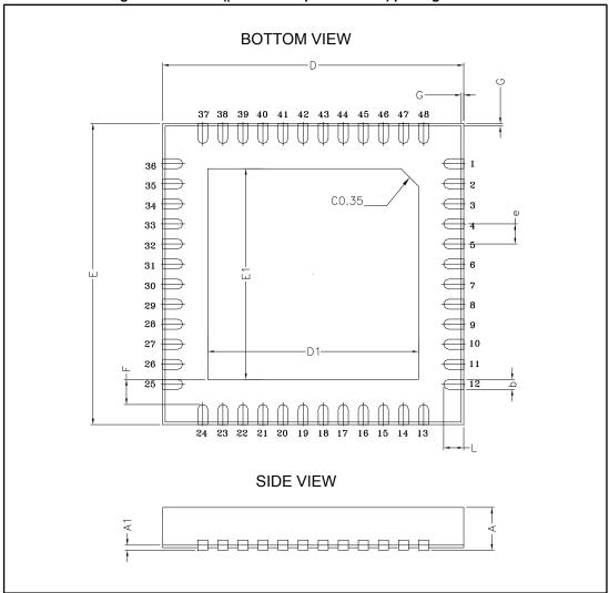
Table 229: QFN48 (|6 x 6 x 0.85 pitch 0.4 mm) mechanical data
