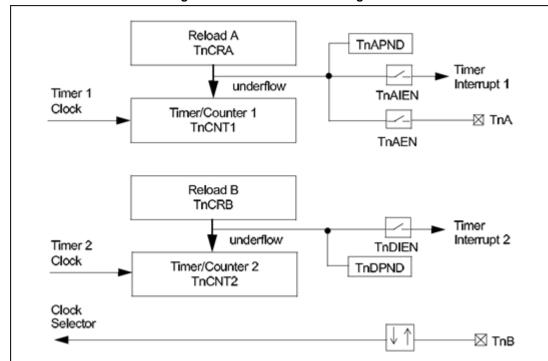
Figure 19: MFT mode 3 block diagram
