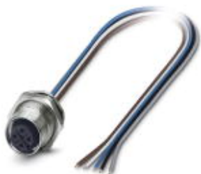
Sensor/actuator flush-type socket, 5-pos., M12 SPEEDCON, A-coded, rear/screw mounting with M16 thread, with 0.5 m TPE litz wire, 5 x 0.34 mm 2
