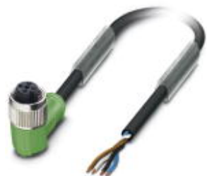
Sensor/Actuator cable, 4-position, PUR halogen-free, black-gray RAL 7021, free cable end, on Socket angled M12, A-coded, Cable length: 10 m
