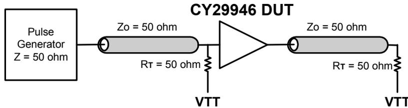
Figure 2. LVCMOS Propagation Delay ( $T_{PD}$ ) Test Reference
