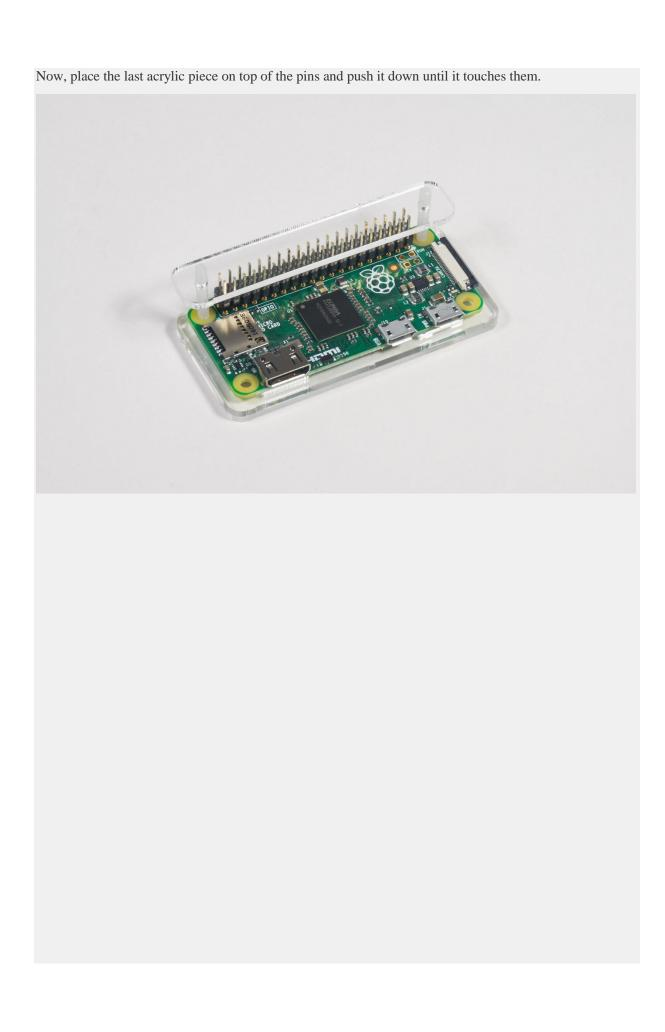
Using a hammer, gently tap back and forth on the top acrylic piece to push the pins through. Pushing one end of the header all the way it can cause the other pins to bend when you hammer them in. It's worth taking your time over this part.
