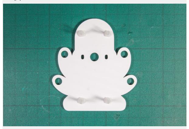
Take the four spacers and slip them onto each of the four bolts. They will space the camera just the right distance away from the Pi Zero W, and the rubber foot (that we'll add later) will prevent too much heat from radiating from the Pi Zero W's CPU to the camera.
