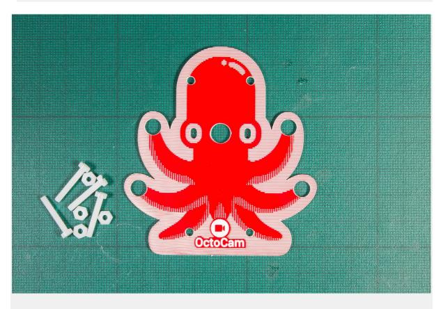
Let's start by taking the red OctoCam mount, the four bolts and four of the nuts. Push each of the four bolts through the circular holes at the top and bottom of the mount, from the front.
