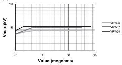
Maximum peak voltage in accordance with "IEC 60065 chapter 14.1" 50 discharges from a 1nF capacitor charged to V max. 12 discharges/minute.
