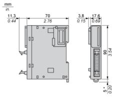
(\*) 8.5 mm/0.33 in. when the clamp is pulled out.
