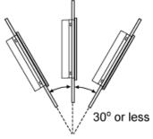
When installing the panel in a slanted position with an incline more than 30°, the ambient temperature must not exceed 40 °C (104 °F). You may need to use forced air cooling (fan,A/C) to ensure the ambient operating temperature is 40°C or less (104 °F or less).
