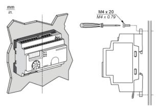
The Access Point is installed according to its vertical axis
