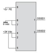
With External Device Monitoring (EDM) feedback loop
