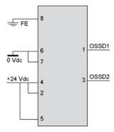
With External Device Monitoring (EDM) feedback loop
