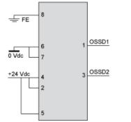
With External Device Monitoring (EDM) feedback loop
