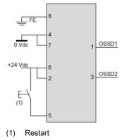
With External Device Monitoring (EDM) feedback loop
