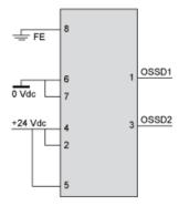
With External Device Monitoring (EDM) feedback loop
