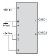
With External Device Monitoring (EDM) feedback loop
