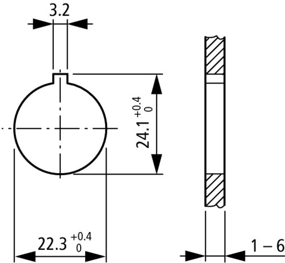
Mounting hole with lug slot
