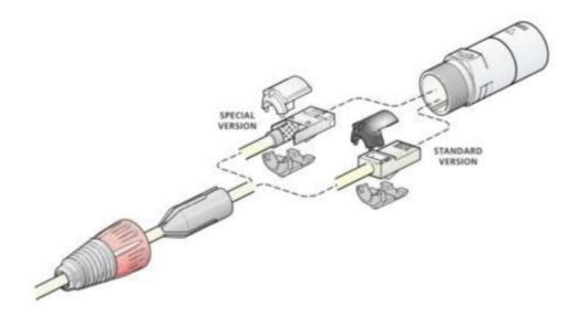
By help of the new alignment system we now support a greater range of RJ45 plugs while in parallel the improved positioning grants a smooth mating with the corresponding etherCON receptacle. Additionally we significantly eased the assembly of the connector since the chuck now clasps around both alignment parts and so it is very convenient to insert the assembly group into the housing.
