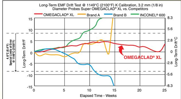
\* Tests conducted using ungrounded probes in an open-air, electric, muffle furnace versus a Type "S", NIST-traceable standard. Individual results may vary depending on customer application. Inconel® is a registered trademark of Special Metals Corporation.
