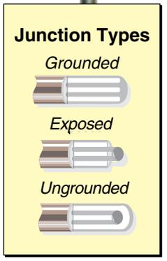
[\*]Specify junction type: **G** (Grounded), **E** (Exposed), **U** (Ungrounded) or **S** (Surface). [\*\*]Specify length in millimeters: 150 mm, 300 mm, 450 mm, or 600 mm. Order standard part number with a suffix “PFA”. Visit [omega.com](http://omega.com) for additional price on 300 mm (12”) probes, 450 mm (18”) probes and 600 mm (24”) probes. 200°C (400°F) max. Note: These diameters will be assembled manually, not molded.
