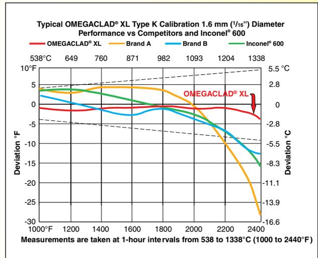
In tests up to 1335°C (2400°F), Super OMEGACLAD® XL outperformed both the Inconel® 600 and other competing high-temperature models.
