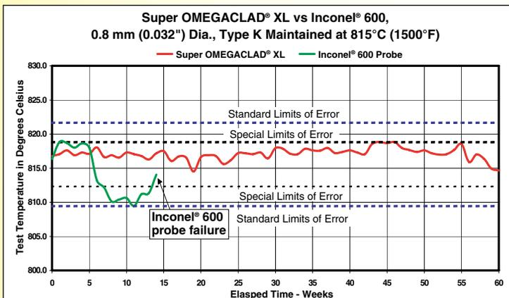
\* Tests conducted using ungrounded probes in an open-air, electric, muffle furnace versus a Type "S", NIST-traceable standard. Individual results may vary depending on customer application. Inconel® is a registered trademark of Special Metals Corporation.
