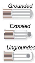
[\*] Specify junction type: **"G"** (Grounded), **"E"** (Exposed), **"U"** (Ungrounded) or **"S"** (Surface). [\*\*] Specify length in inches: **6, 12, 18 or 24**.
