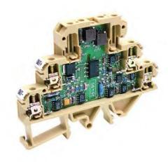
The picoPak™ I-I is a very compact isolator for 4-20mA loops. The output is loop powered. The module is perfect for eliminating ground loops and providing increased protection for PLC and DCS analog inputs.
