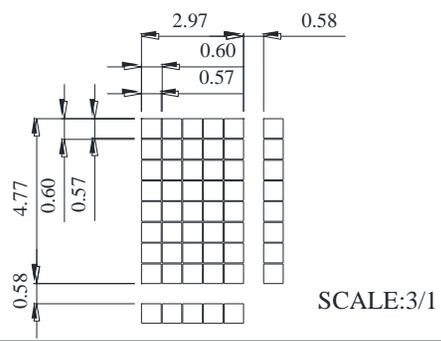
The non-specified tolerance of dimension is ±0.3mm.
