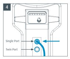
Plug in the 10m Push Fit 'F' to 'F' Flexible Cable to The cable connection port. See page 14 for receiver end connections.
