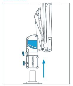
We recommend removing unit when not in use. Loosen azimuth lock knob and lift system.
