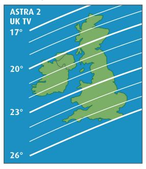
Use the elevation map to find the required elevation for your area
