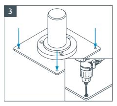
Using mechanical fixings (recommended if travelling before flexible adhesive has properly cured).
