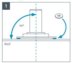
We strongly recommend mounting on the centre line of your boat. For correct performance, the nylon mount must be vertical.
