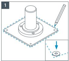
Mark out position of mount on roof and place at least 1 washer into each corner of marked out area.
