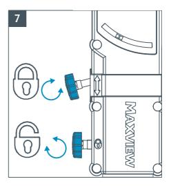
Once satellite is located, lock off the rotation by turning Azimuth lock knob. If you are experiencing signal drop out, fine tune your signal by slightly adjusting the elevation to improve TV picture quality. Again, you can aid this process by using:
