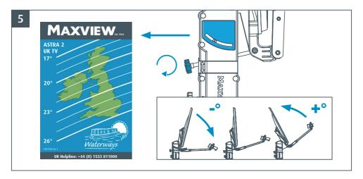
Use the elevation map to determine the required angle for your location. Set the dish to this angle using the elevation knob and indicator.
