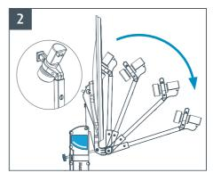
Pull down LNB arm from magnetic lock.
