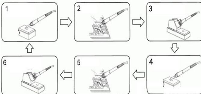
1. Before soldering, clean the tip on sponge, and then wear tin on the tip - Start your soldering work - when not in use (during breaks), please put the soldering iron on the holder -à clean the tip, wear tin on the tip - do the soldering - vice versa..
