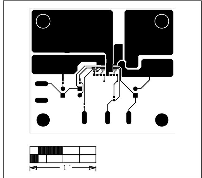
MAX17531 5V EV Kit (μMAX) PCB Layout—Component Side
