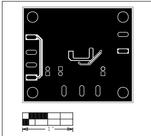
MAX17531 5V EV Kit (μMAX) PCB Layout—Solder Side
