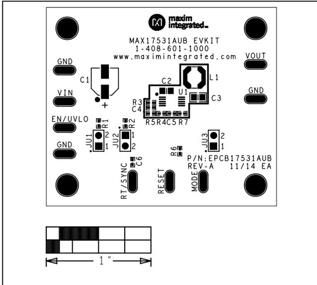
MAX17531 5V EV Kit (μMAX) Component Placement Guide—
