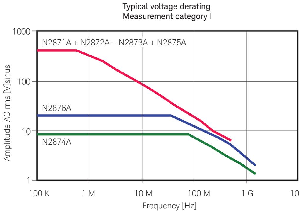
Figure 9. N2870A Series amplitude vs. frequency characteristics.
