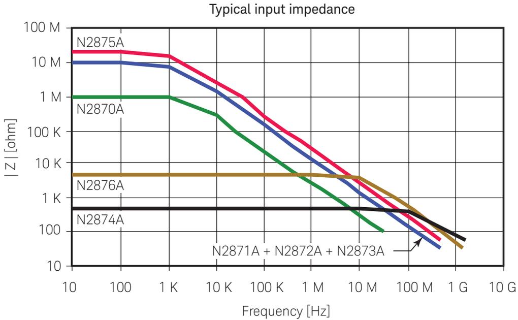
Figure 10. N2870A Series input impedance vs. frequency characteristics.
