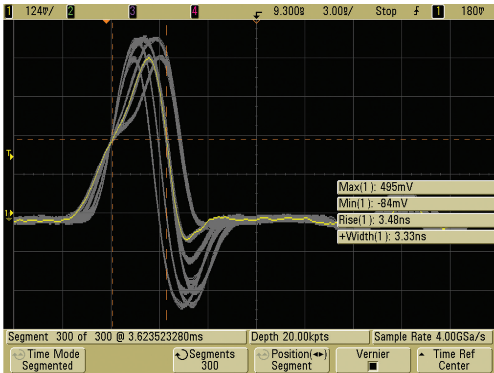
Figure 1. Segmented memory acquisition captures 300 consecutive laser pulses for analysis.
