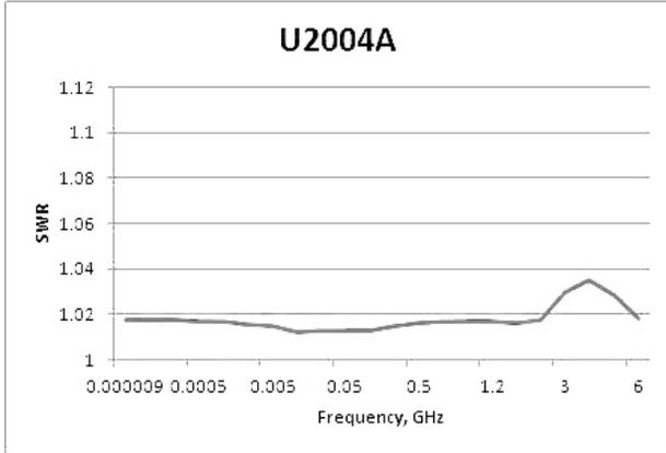
Typical SWR for U2004A sensor (25 °C ± 10 °C)
