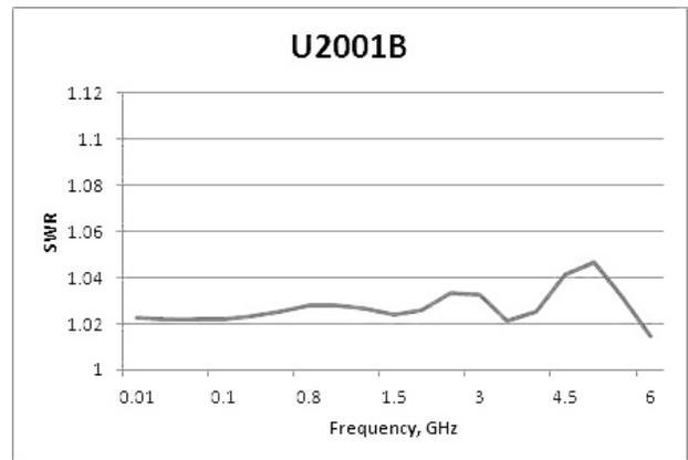
Typical SWR for U2001B sensor (25 °C ± 10 °C)
