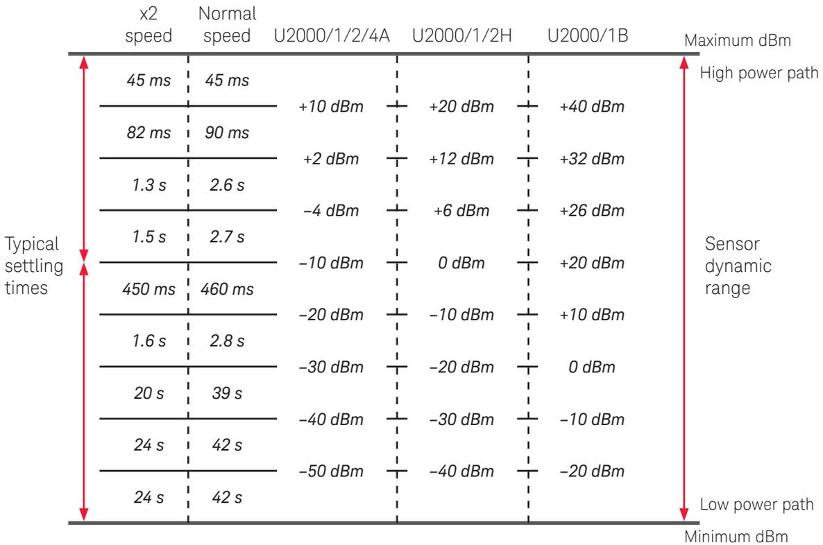
Settling time with auto filter, default resolution, and a 10 dB decreasing power step (not across the switching point)
