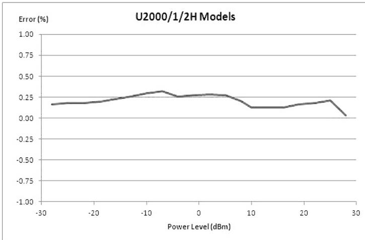
1. Measurement uncertainty  $\leq 1.9\%$ . At room temperature and excluding power level dependent terms (zero set, drift, and noise). Refer to Keysight Fundamentals of RF and Microwave Power Measurements (Part 3) Power Measurement Uncertainty per International Guide (Application Note 1449-3), 5988-9215EN for more information on measurement uncertainty.
