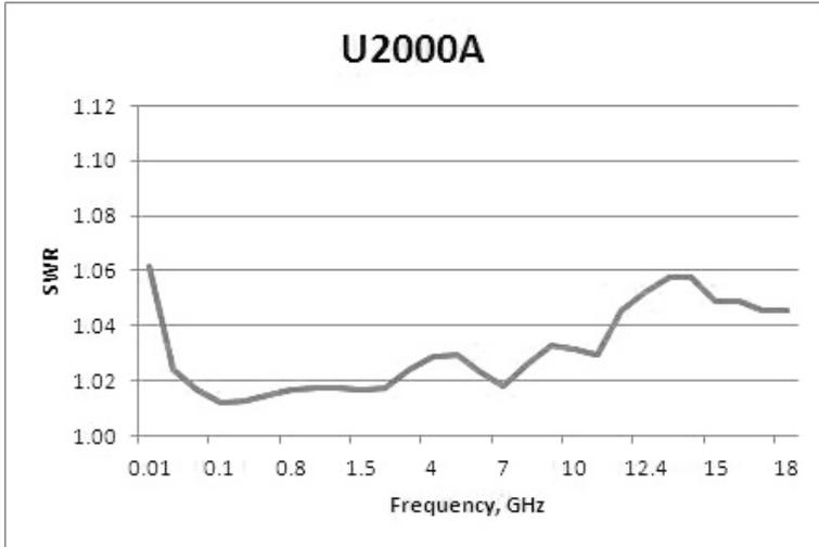
Typical SWR for U2001A sensor (25 °C ± 10 °C)
