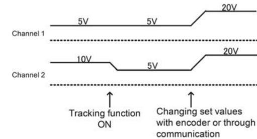
The tracking function is available on the dual output model (PSB-2400L2) only. It allows the setting of both channels to be changed at the same time. When the value of the one channel is changed, and the other channel will automatically change its value accordingly if the tracking function is active (ON).
