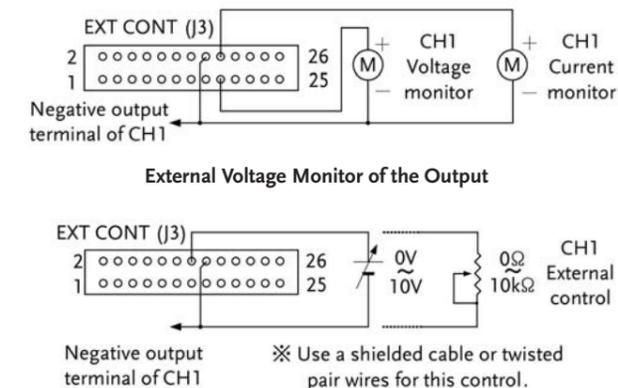
External Voltage Control of the output
