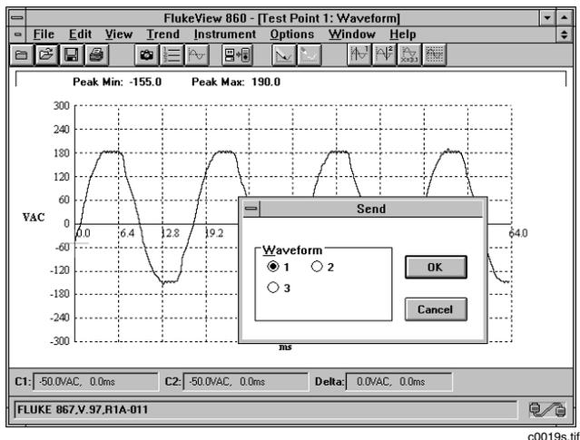
**Figure 19. Sending a Waveform to GMM Memory**
