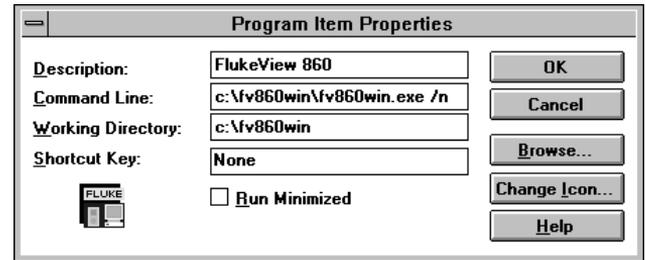
Figure 4. Using the /n Command Line Switch
