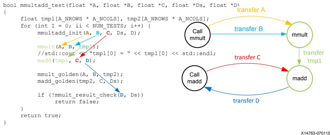
Because the intermediate array variable `tmp1` is used only to pass data between the two hardware functions, the `sdscc` system compiler chains the two functions together in hardware with a direct connection between them.
