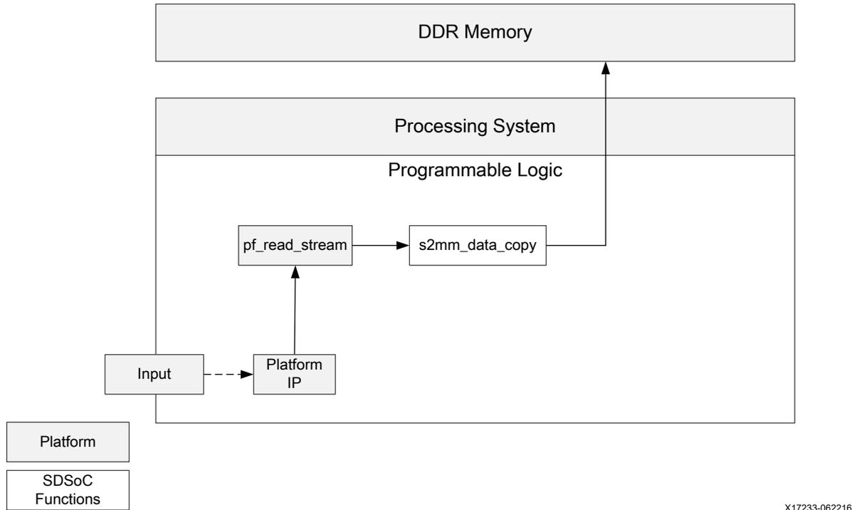
In this example, the `zc702_axis_io` platform proxies actual I/O by providing a free-running binary counter (labeled Platform IP in the diagram) running at 50 MHz, connected to an AXI4-Stream Data FIFO IP block that exports an AXI4-Stream master interface to the platform clocked at the data motion clock (which might differ from the 50 MHz input clock).
