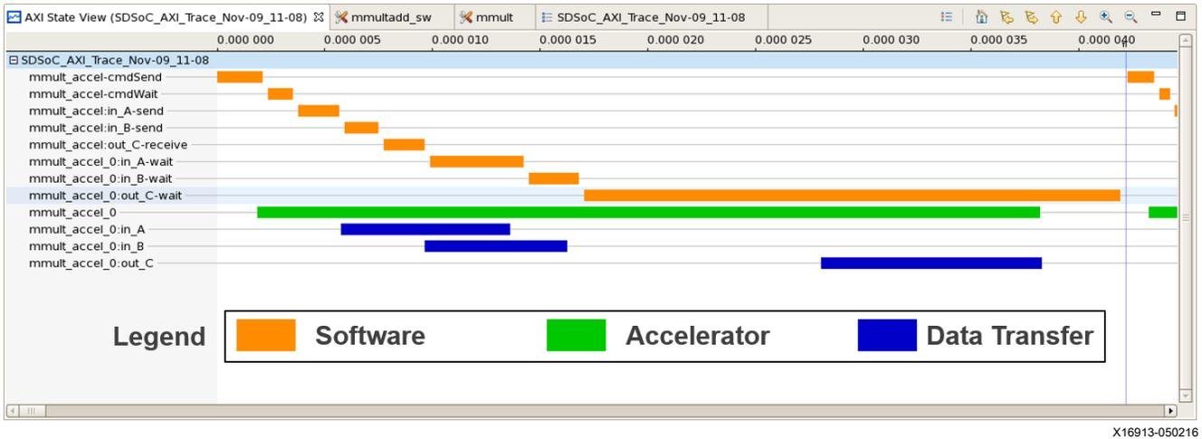
Each trace event has a few different attributes: name, type, start time, stop time, and duration. This data is shown as a tool-tip when the cursor hovers above one of the event rectangles in the view.
