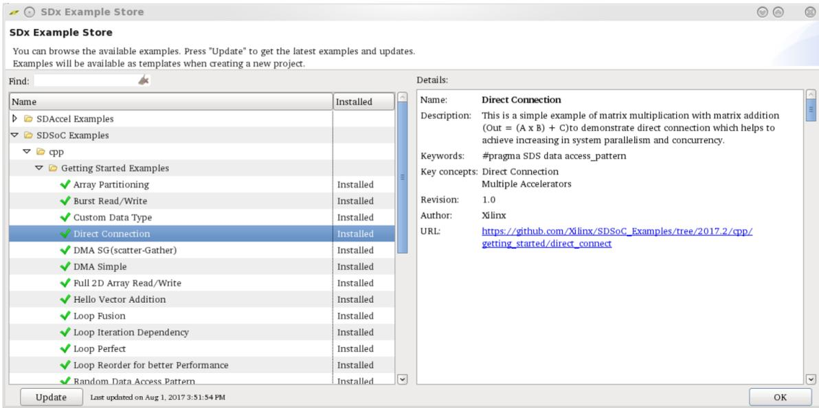
The GitHub examples also indicate if they are installed or not. Use the **Refresh** button to ensure you have the latest update from the repository. Click **Install** to download and install the example design.
