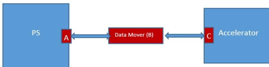
Without any SDS pragma, the SDSoC environment generates the data motion network based on an analysis of the source code. However, the SDSoC environment also provides pragmas for you to guide the data motion network generation.
