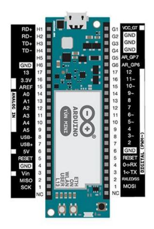
Atheros AR9331 pins: Each of these pins can be used by LininoOS side as peripherals of Linux Kernel. In addition, some pins have specialized functions:
