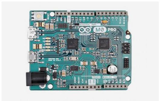
The Arduino M0 Pro is an Arduino M0 with a step-by-step debugger.
