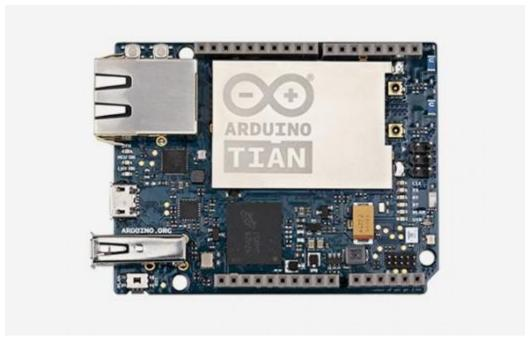
The Arduino Tian unleashes the power of a small computer running Linux connected to a 32-bit microcontroller.
