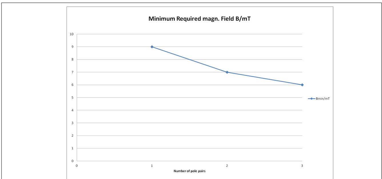
**Figure 8 Minimum magnetic field  $B$  for different numbers of pole pairs @  $B_m = -1\text{mT}$**
