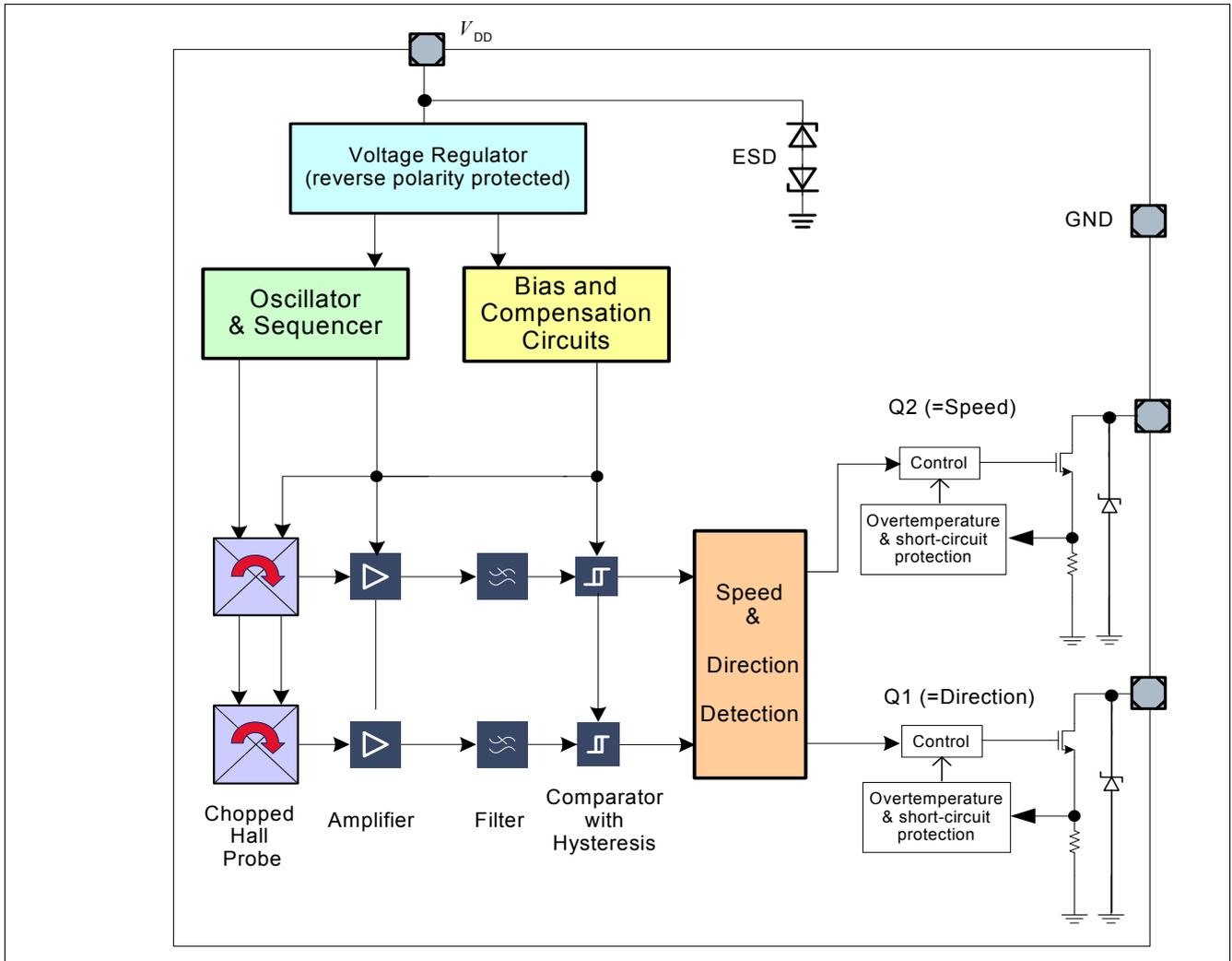
**Figure 2** Block diagram of the TLE4966V-1K
