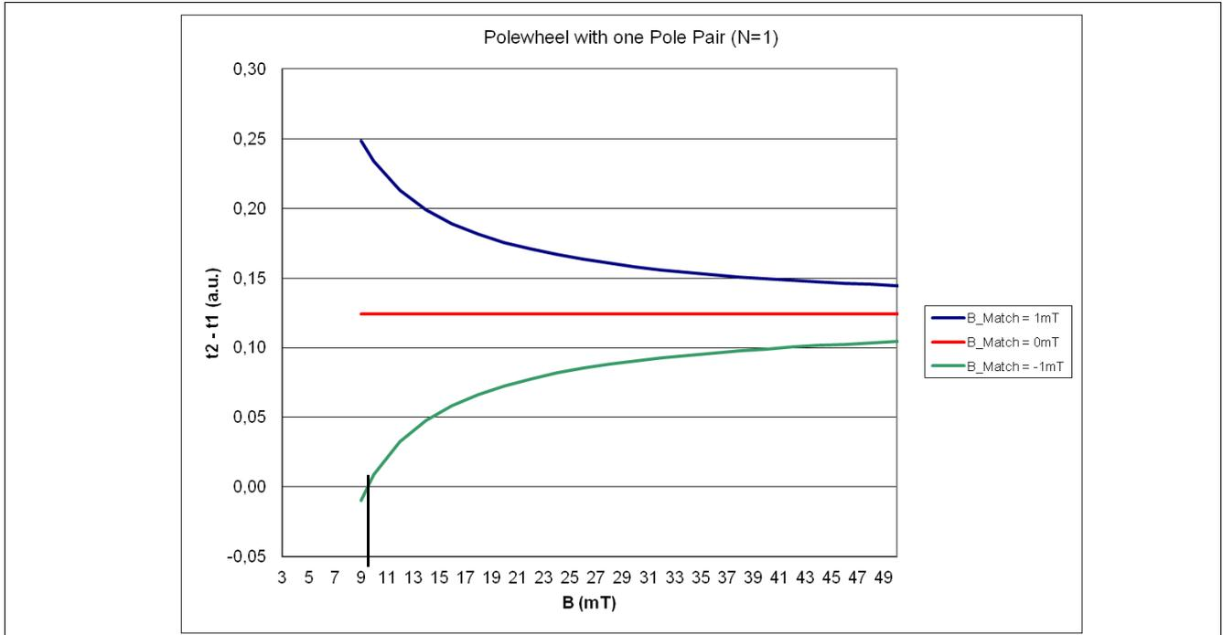
Figure 5 Pole wheel with N = 1, Minimum required field  $B_{min} = 9mT$  for  $t_2 - t_1 = 0$
