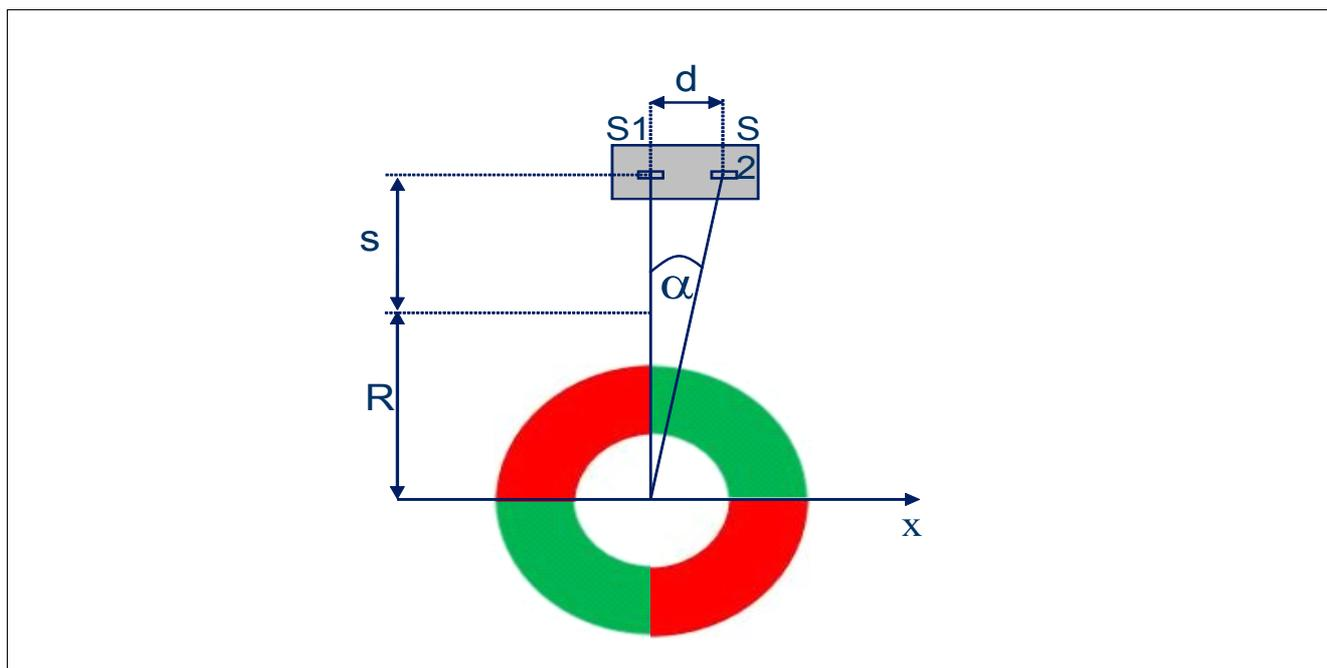
**Figure 1 Configuration with pole wheel and TLE4966V-1K double Hall sensor**
