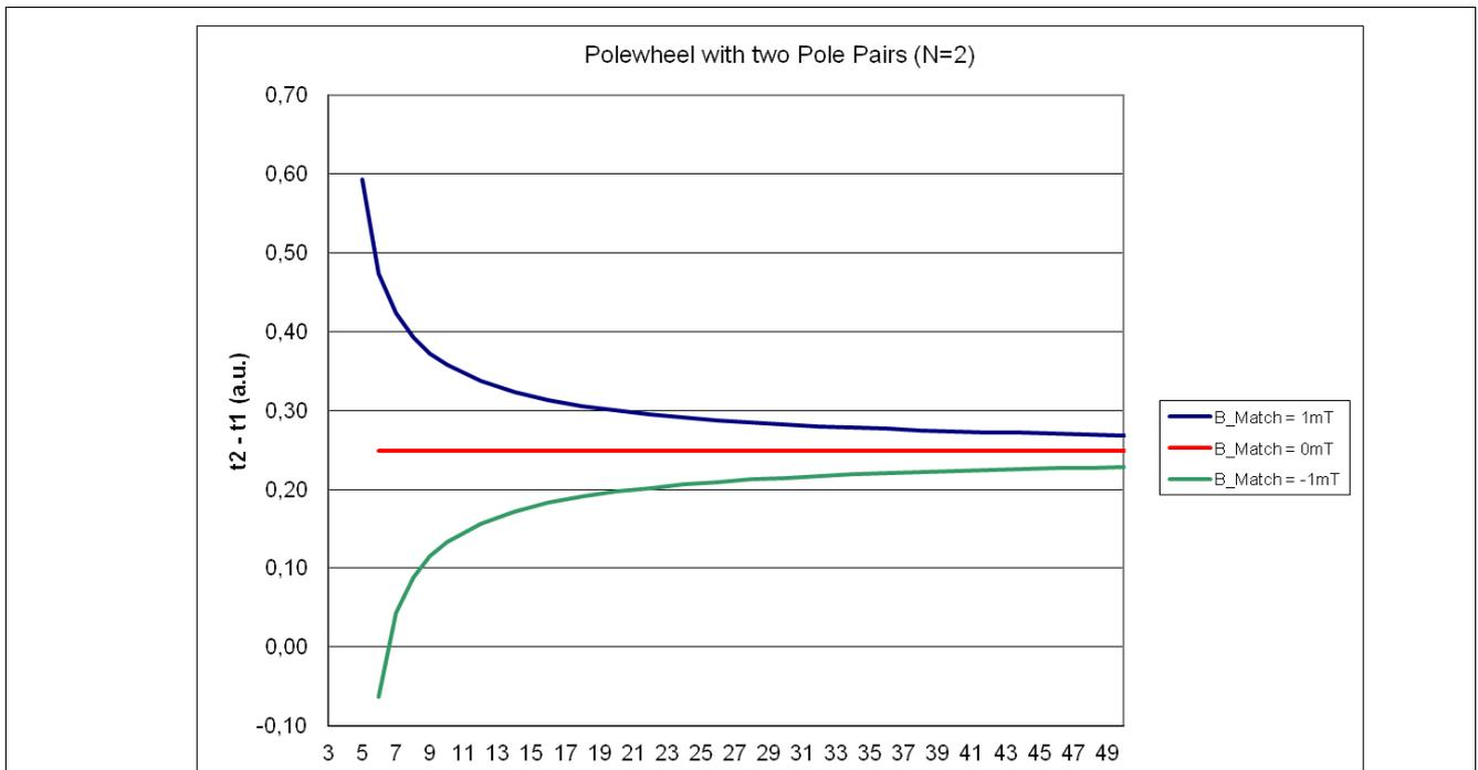
Figure 6 Pole wheel with N = 2, Minimum required field  $B_{min} = 7mT$  at  $t_2 - t_1 = 0$
