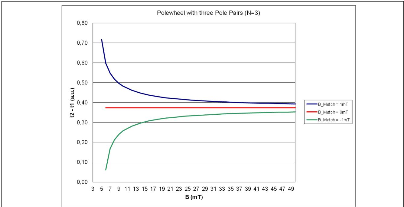
**Figure 7 Pole wheel with N = 3, Minimum required field  $B_{min} = 6 \text{ mT}$  at  $t_2 - t_1 = 0$**
