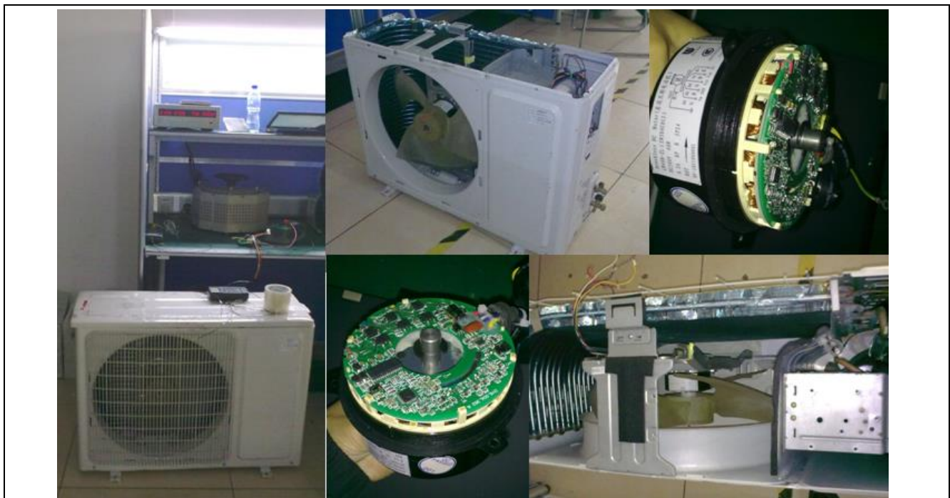
Figure 6 Commercial air-conditioning split system, showing the motor drive card housed on the back of the BLDC fan motor
