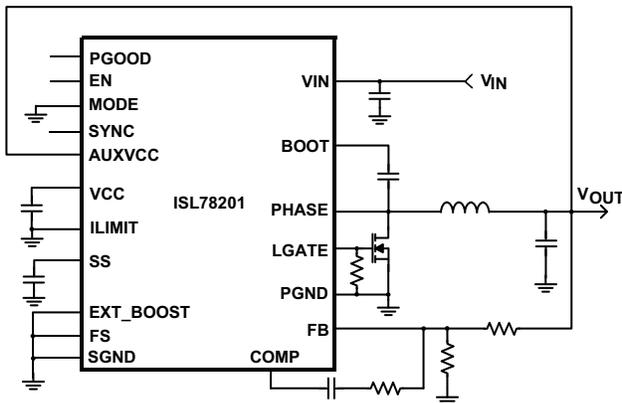
FIGURE 5A. SYNCHRONOUS BUCK
