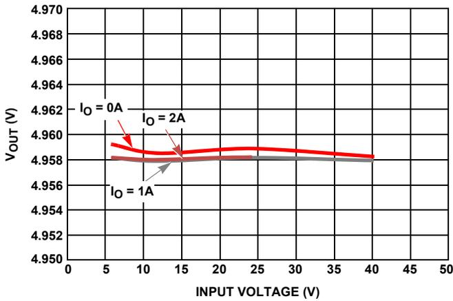
FIGURE 9. LINE REGULATION,  $V_{OUT}$  5V,  $T_A = +25^\circ\text{C}$
