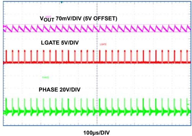
FIGURE 23.  $V_{IN}$  24V, 80mA LOAD, PFM MODE
