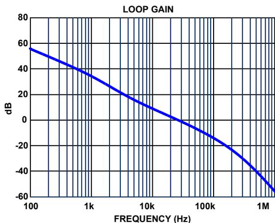
FIGURE 37. SIMULATED LOOP BODE PLOT
