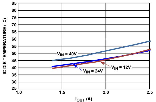
FIGURE 16. IC DIE TEMPERATURE UNDER +25°C AMBIENT TEMPERATURE, STILL AIR, 500kHz, V<sub>OUT</sub> = 9V
