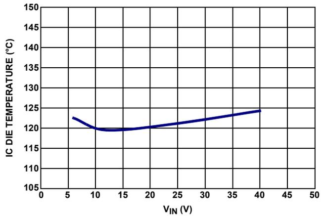
FIGURE 14. IC DIE TEMPERATURE UNDER +105°C AMBIENT TEMPERATURE, 100 CFM, 500kHz, V<sub>OUT</sub> = 5V, I<sub>O</sub> = 2A
