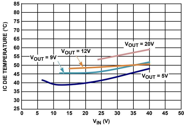
FIGURE 15. IC DIE TEMPERATURE UNDER +25°C AMBIENT TEMPERATURE, STILL AIR, 500kHz, I<sub>O</sub> = 2A
