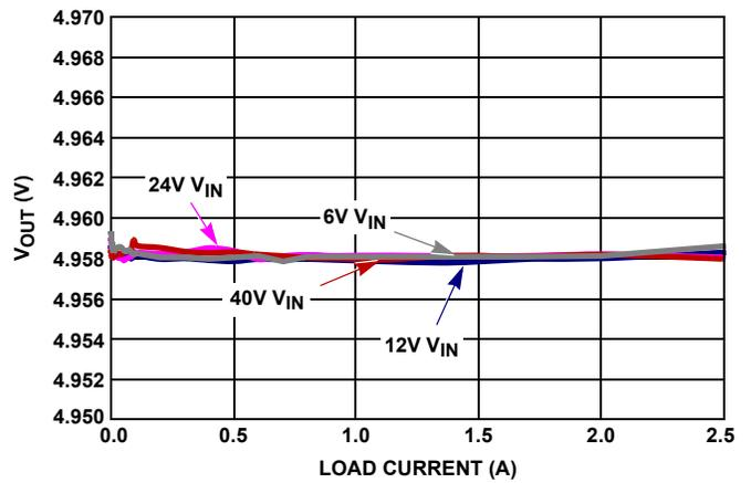
FIGURE 10. LOAD REGULATION,  $V_{OUT}$  5V,  $T_A = +25^\circ\text{C}$
