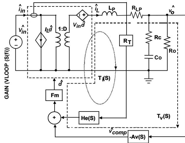
FIGURE 35. SMALL SIGNAL MODEL OF BUCK REGULATOR
