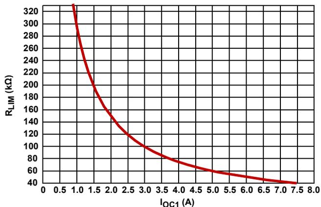
FIGURE 34. R<sub>LIM</sub> vs I<sub>OC1</sub>
