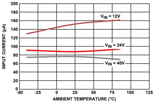
FIGURE 13. INPUT QUIESCENT CURRENT UNDER NO LOAD, PFM MODE, AUXVCC CONNECTED TO V<sub>OUT</sub>. V<sub>OUT</sub> = 5V
