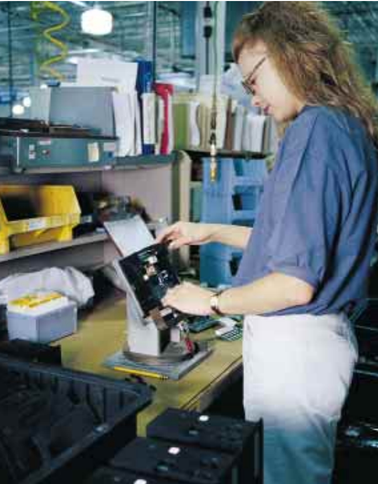
Component leads are formed prior to insertion into PCBs.
