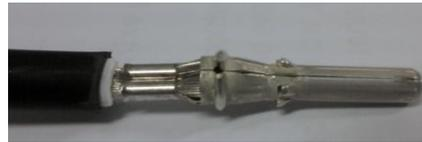
Closed barrel pin S&F contact
