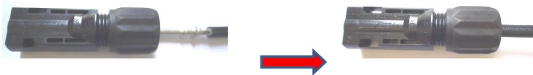
Back cap must be closed using a torque between 2.6 and 2,9NM.
