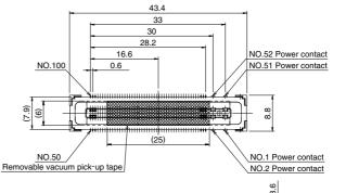
(PCB thickness: 1 mm min.)
