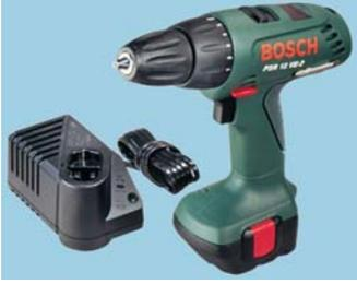
12V drill/driver with electronic speed control, variable speed and smooth acceleration. Rotary action for drilling metal, wood, plasterboard and breeze block. Single sleeve keyless chuck and automatic spindle lock. Two mechanical gears deliver maximum torque at low speeds. Supplied with charger, 2 x battery packs and carry case.
