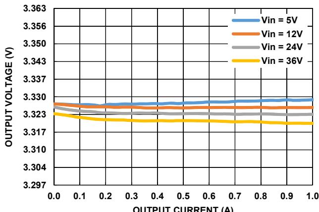
FIGURE 19.  $V_{OUT}$  REGULATION vs LOAD, PWM,  $V_{OUT} = 3.3\text{V}$
