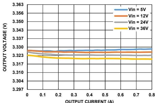
FIGURE 31.  $V_{OUT}$  REGULATION vs LOAD, PWM,  $V_{OUT} = 3.3\text{V}$
