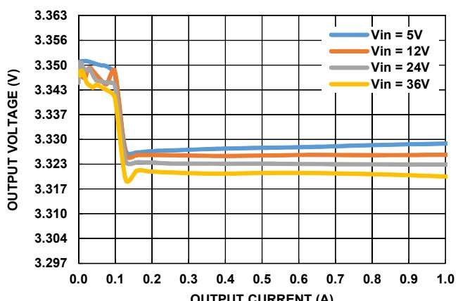
FIGURE 20.  $V_{OUT}$  REGULATION vs LOAD, PFM,  $V_{OUT} = 3.3\text{V}$
