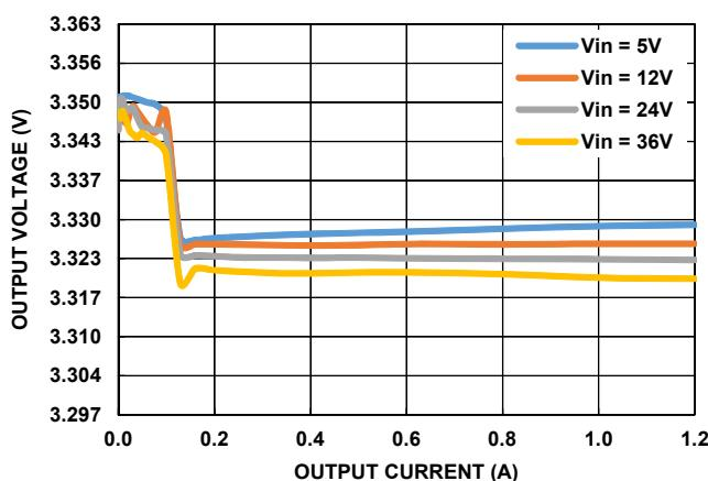
FIGURE 25.  $V_{OUT}$  REGULATION vs LOAD, PFM,  $V_{OUT} = 3.3\text{V}$
