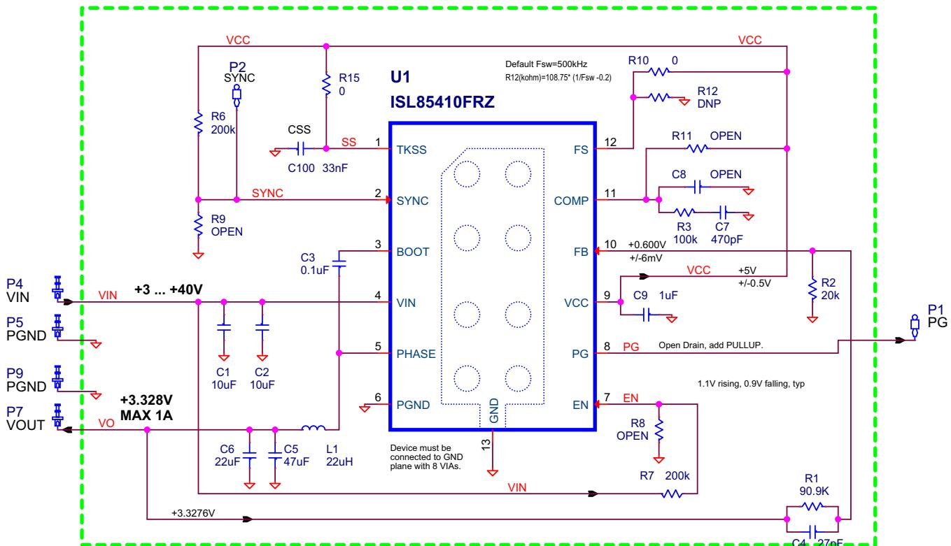
NOTE: The input electrolytic capacitor  $C_{10}$  is optional and it is used to prevent transient voltages when the input test leads have large parasitic inductance. It can be removed if the IC is used in a system application.
