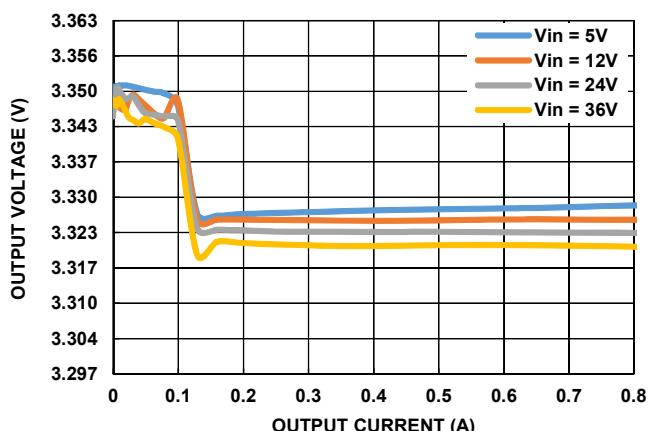
FIGURE 32.  $V_{OUT}$  REGULATION vs LOAD, PFM,  $V_{OUT} = 3.3\text{V}$
