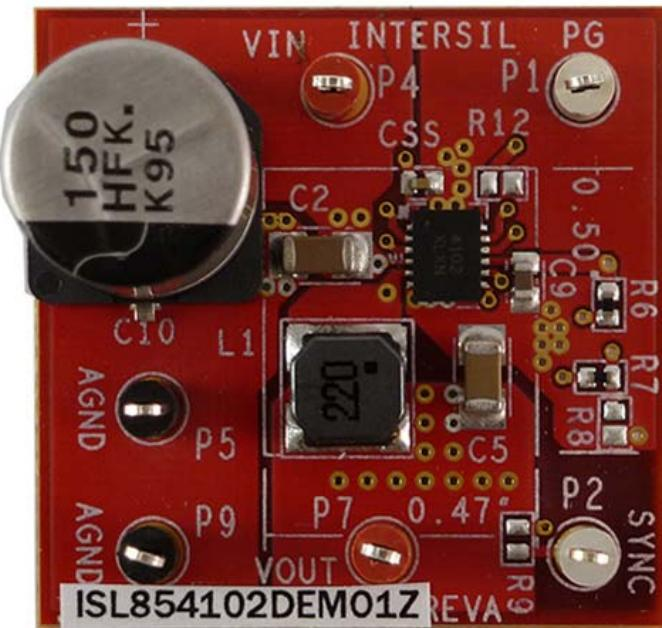
FIGURE 4. ISL854102DEMO1Z DEMONSTRATION BOARD (TOP)
