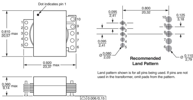
Figure 3. Typical Dimensional Drawing
