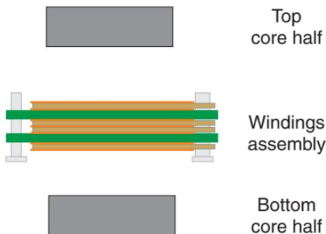
Figure 1. Major Components of a Planar Transformer
