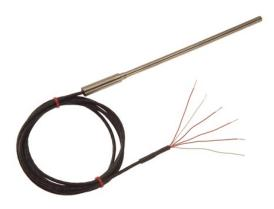
Duplex PRT's with two independent PT100 detectors inside tip of probe. This allows one probe to be connected to two measurement or control devices; alternatively, one sensor may be used as a primary and the other as a backup, eliminating the need to remove and replace the probe if one of the sensors should fail.
