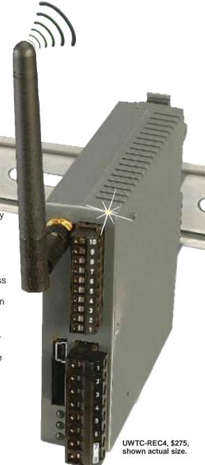
Note: The UWTC-REC4 can be powered directly by the PLC or data logger you are connecting to and will not require an additional power source if the instrument has 12 to 24 Vdc @ 250 mA available for external devices. If your instrument does not have a power source available for external devices you will need to add an additional power supply (iDRN-PS-1000, \$150) to power the wireless receiver. This power supply can power up to 3 UWTC-REC4 receivers. Visit omega.com/wireless for more
