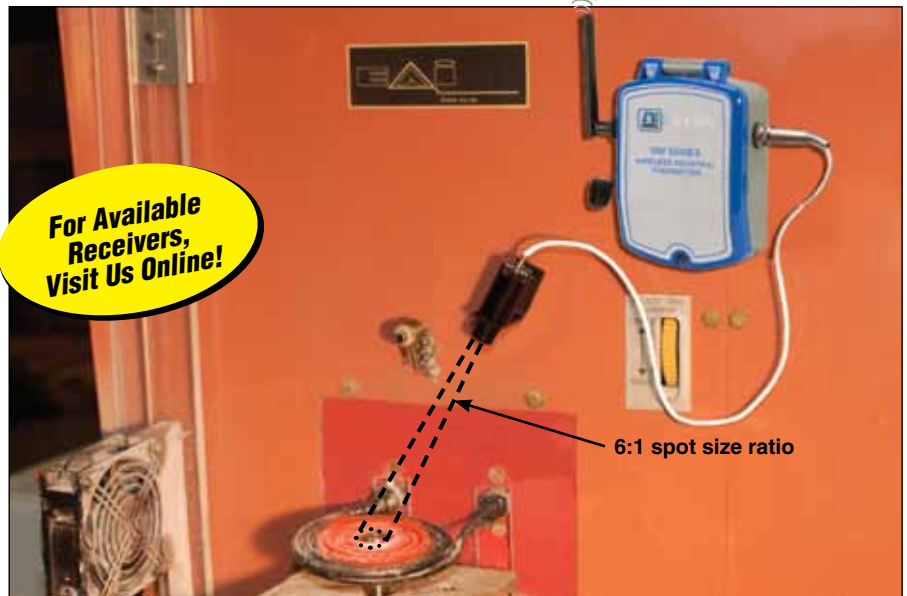
Monitoring temperature of heating coil on an induction welder.
