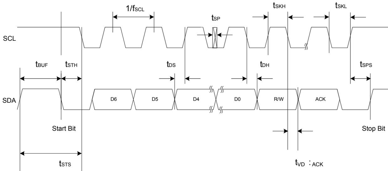
**Figure 1.1. I<sup>2</sup>C Interface Timing**
