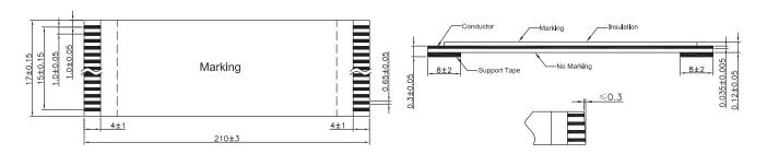
Pitch 1mm FFC 16 Core (Pin) Cable
