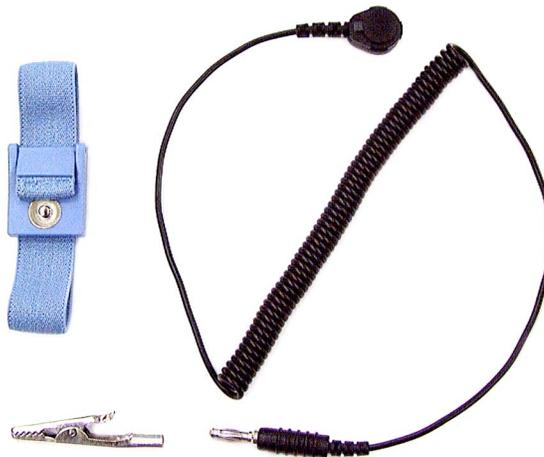
This economy wrist strap set features a fully adjustable stretch fabric wristband and 6ft coiled cord. The band provides 360 degree conductivity around the wrist. Band curling is reduced by the woven band fabric. The retractable coil cord connects to the wrist band via a 4mm snap and contains a 1 megohm resistor. A "spinning style" banana jack reduces cord tangles and improves the cord's life span. Includes alligator clip.
