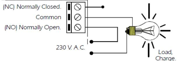
During the operating, and according to its load, it is possible that a fluctuation appear and/or an incorrect output operating. If it is the case, you have to install a circuit against sparks (resistor or capacitor) between both relay contacts used for the connection. (see the drawing)
