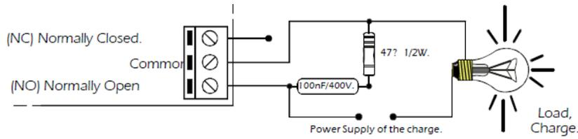
**INSTALLATION.** You have to use shielded cable for all connections and connect ground to the chassis of the box. Maintain a correct distance with other modules as power stage, which could dissipate a big heat. Install the module in a metallic enclosure with a ventilation grille .
